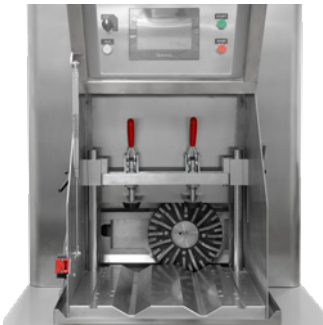
Detail of the grinding chamber with automatic cradle
